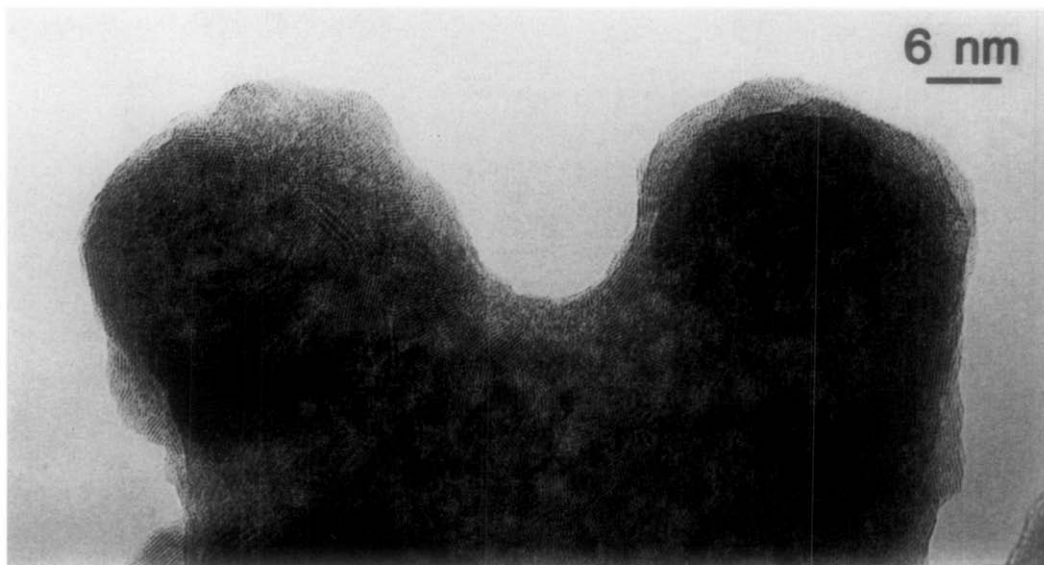
FIG. 14. A small section of a precipitate having snowflake morphology is seen in this high-magnification image to consist of sintered polycrystalline spheres.
