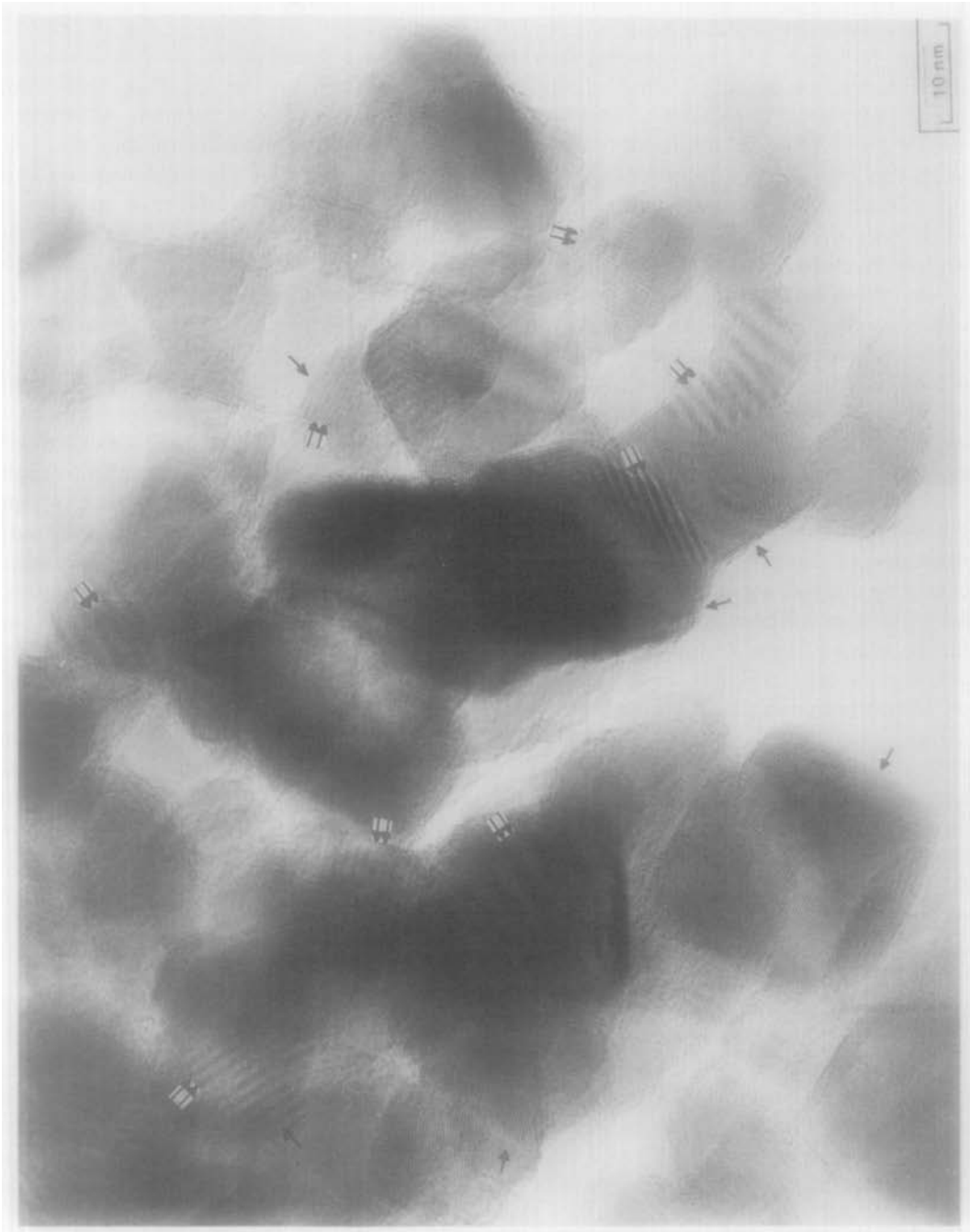
FIG. 5. A typical field of view of P25 particles. Lattice fringes (single arrow) and Moiré patterns (double arrows) are indicated. The fact that overlapping crystallites show fringe contrast indicates that many are plate-like.
