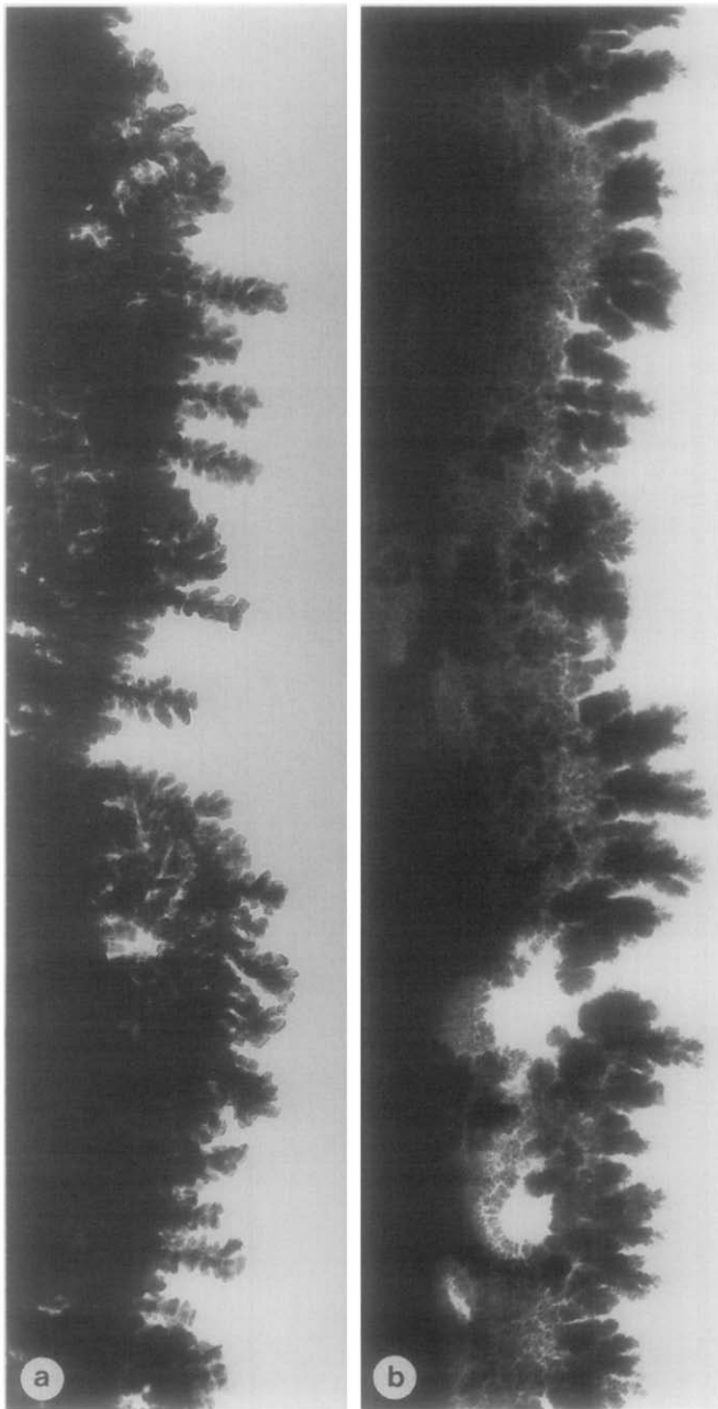
FIG. 5. Series of four surface profiles for increasing electrolysis periods. Note isolated dendrite trees (a), impinging trees (b), coarsening (c), and development of quasiperiodic compacted crystallites in (d).
