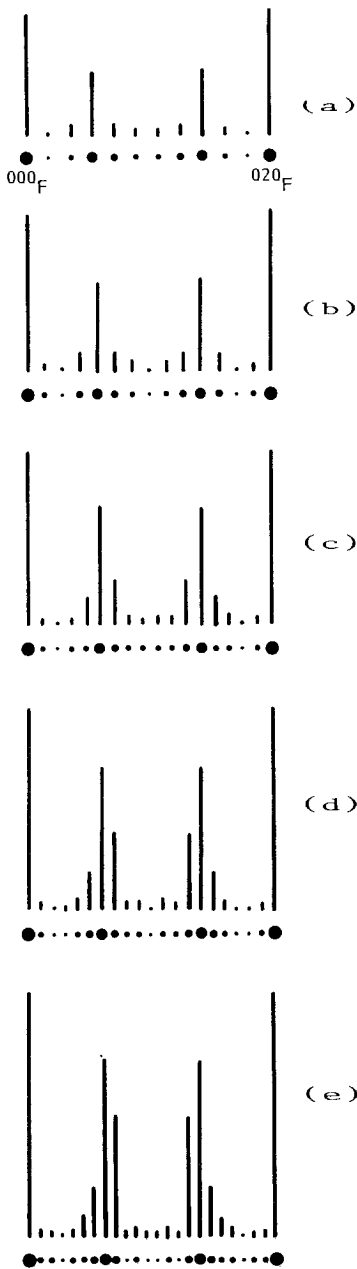
FIG. 6. Calculated intensities for the superlattice spots lying between the 000 and 020 subcell reflections for the sequences (a) \{4^23^1\} ( L = 11 ); (b) \{4^23^2\} ( L = 14 ); (c) \{4^23^3\} ( L = 17 ); (d) \{4^23^4\} ( L = 20 ); (e) \{4^23^5\} ( L = 23 ). In each part of the figure, the intensities of the reflections, represented as vertical lines, are shown above a schematic illustration of the distribution and intensities of the reflections.
