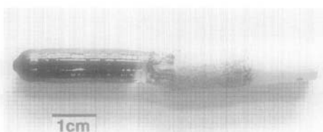
FIG. 1. As-grown SrTiO_{2.98} single crystal.
