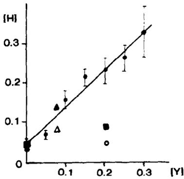
FIG. 1. Hydrogen concentration [H], moles of atoms per mole of oxide, as a function of the dopant concentration [Y], moles of atoms per mole of oxide in  $\text{BaCe}_{1-y}\text{Y}_y\text{O}_{3-\delta}$ : ● ceramics, prepared by cation precipitation from solution; ○ ceramics after thermal treatment in vacuum. ■ induction melting; and in  $\text{SrCe}_{0.92}\text{Dy}_{0.08}\text{O}_{3-\delta}$ : ▲ ceramics, △ ceramics after treatment in vacuum.
