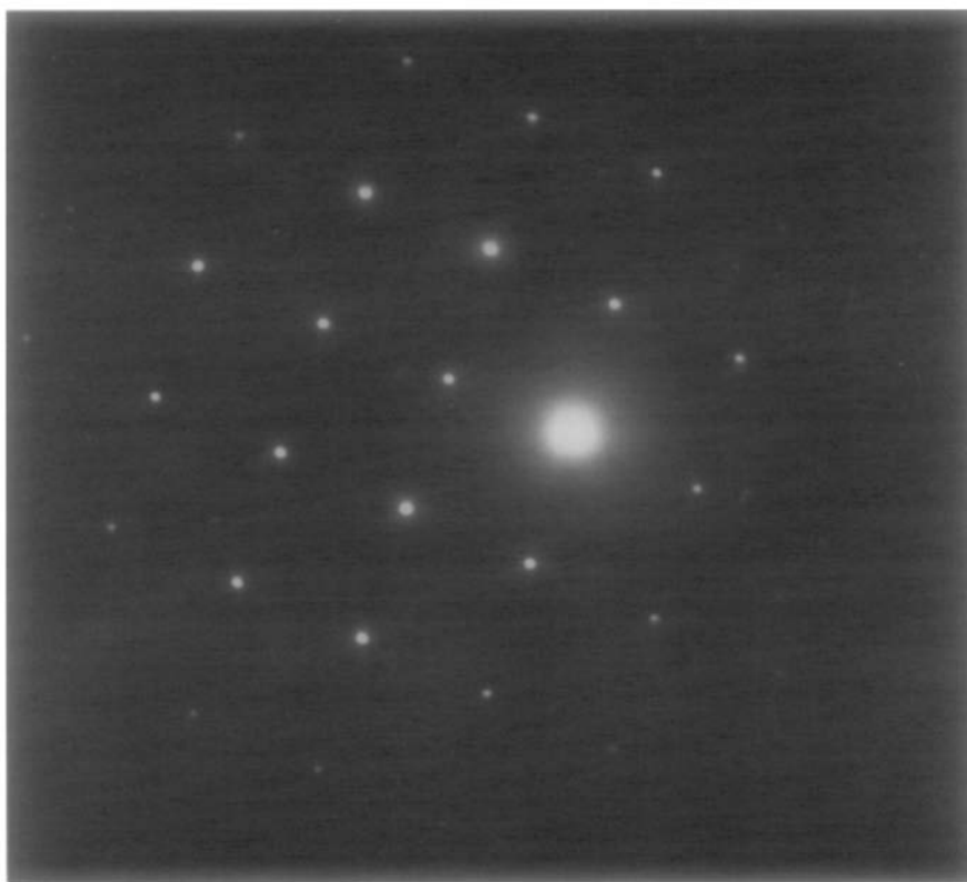
FIG. 2. Selected area diffraction pattern of \text{NdSrNiO}_{4-x}\text{F}_y crystallite ([111] zone axis).
