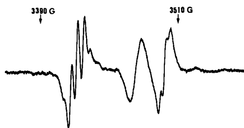
FIG. 3. A 120 K, [\bar{1}10] EPR spectrum of the \text{Cr(V)} species thermally produced in (\text{NH}_4)_2\text{SnCl}_6 . The microwave frequency was about 9.5 GHz (same for the other figures).
