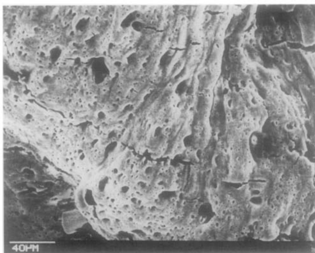
FIG. 2. SEM micrograph of as prepared \text{Ni}_{0.5}\text{Zn}_{0.5}\text{Fe}_2\text{O}_4 foam prepared by combustion method.
