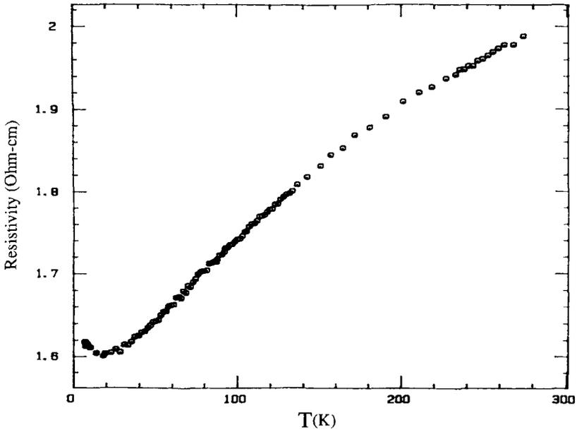
FIG. 5. Temperature dependence of the electrical resistivity of a polycrystalline sample of  $\text{Ca}_3\text{BiN}$ .
