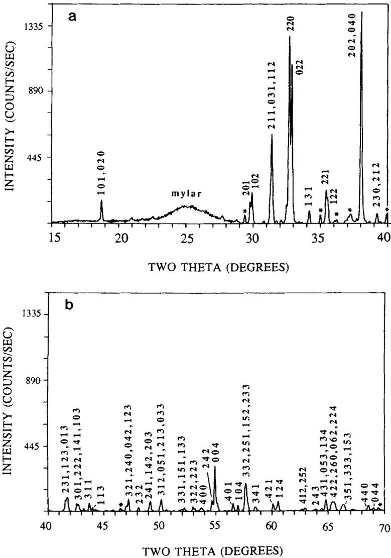
FIG. 2. X-ray powder diffraction pattern of  $\text{Ca}_3\text{PN}$ . The pattern is indexed on an orthorhombic cell; the broad peak at  $25^\circ$  is from a flat mylar covering over the air-sensitive sample. Impurities or second phases are indicated by \*.
