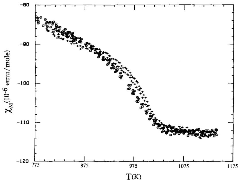
FIG. 3. Magnetic susceptibility of  $\text{Ca}_3\text{AsN}$  at high temperatures. Two curves are shown: one was taken on heating ( $\odot$ ), the other one is a cooling curve ( $+$ ); both were taken at a rate of 100 K/hr. A phase transition at 1025 K with a small hysteresis is implied for  $\text{Ca}_3\text{AsN}$ .
