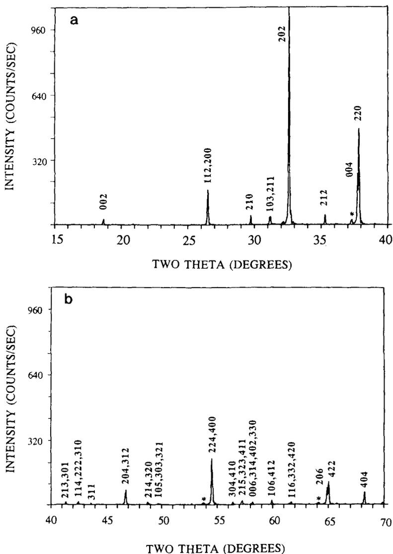
FIG. 1. X-ray powder diffraction pattern of  $\text{Ca}_3\text{AsN}$ . The pattern is indexed on a tetragonal cell, but the true symmetry is orthorhombic with  $a$  and  $b$  almost the same (see Table I). Asterisk signs, \*, are used to indicate impurities or second phases. The air-sensitive sample was covered by a thin layer of mylar for protection, but the mylar formed a semicircular arc over the sample so that there were no diffraction peaks from the mylar.
