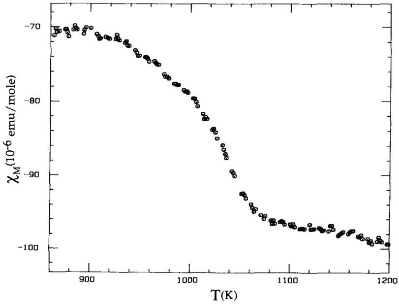
FIG. 4. High temperature magnetic susceptibility of  $\text{Ca}_3\text{PN}$ . A phase transition at 1070 K is also implied for  $\text{Ca}_3\text{PN}$ .
