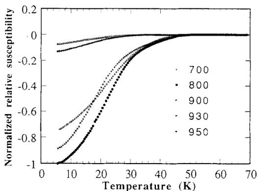
FIG. 4. Temperature dependence of the normalized relative susceptibility [taking the limiting, low temperature (5 K) value as  $-1$  for the sample annealed at 800°C] of the powdered  $(\text{Pb}_{0.7}\text{Cu}_{0.3})\text{Sr}_2(\text{Ca}_{0.5}\text{Y}_{0.5})\text{Cu}_2\text{O}_{7+\delta}$  samples annealed at the temperatures of 700, 800, 900, 930, and 950°C.
