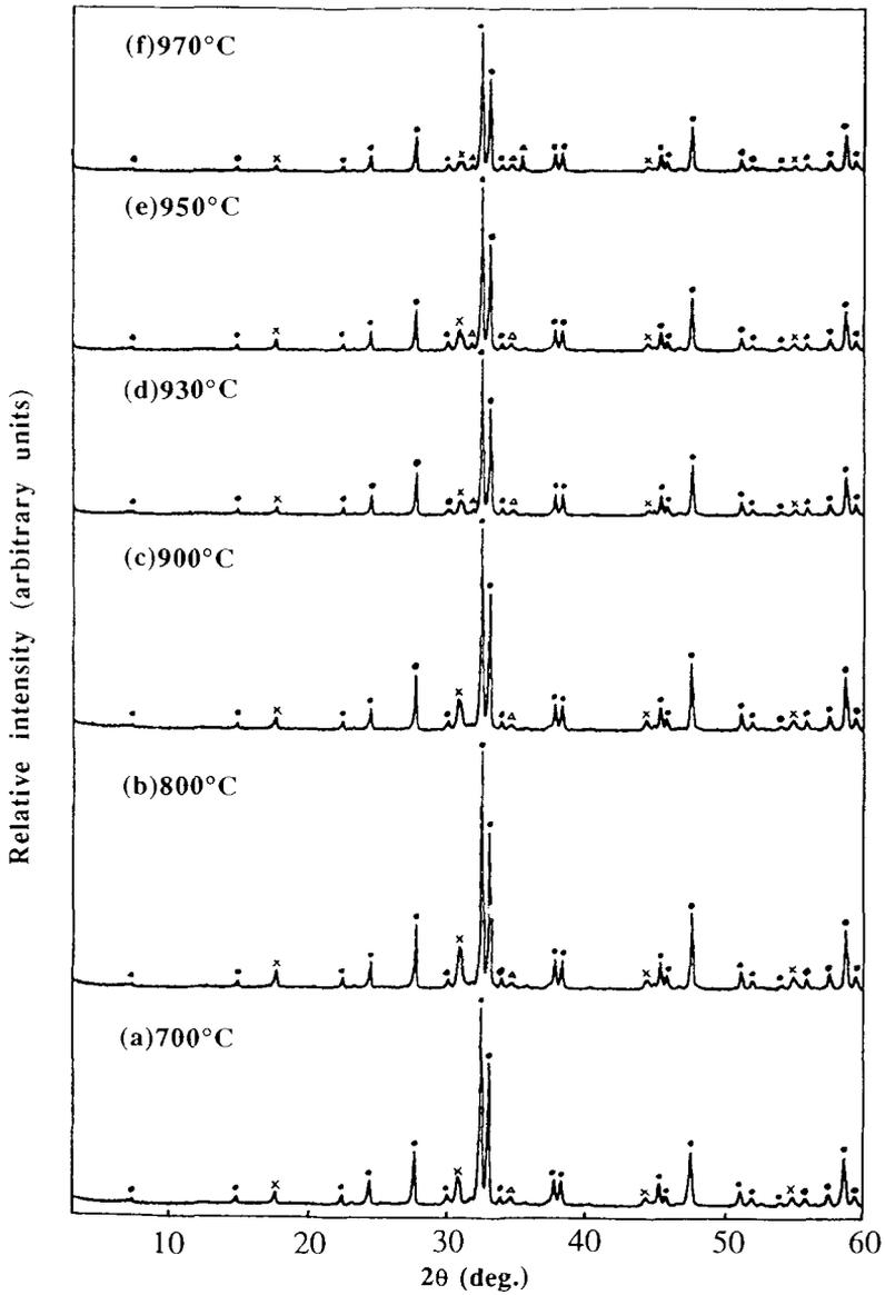
FIG. 1. Powder XRD patterns of the  $(\text{Pb}_{0.7}\text{Cu}_{0.3})\text{Sr}_2(\text{Ca}_{0.5}\text{Y}_{0.5})\text{Cu}_2\text{O}_{7-\delta}$  samples annealed at the temperatures of (a) 700°C, (b) 800°C, (c) 900°C, (d) 930°C, (e) 950°C, and (f) 970°C. A tetragonal superconducting phase labeled by "●," an impurity hexagonal phase labeled by "×," and an unidentified impurity phase labeled by "△" are also shown.
