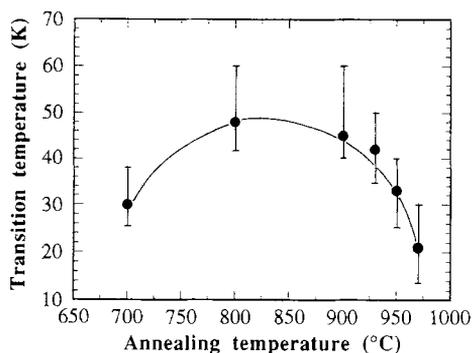
FIG. 3. Summarization of the characteristic superconducting properties (derived from Fig. 2) for the  $(\text{Pb}_{0.7}\text{Cu}_{0.3})\text{Sr}_2(\text{Ca}_{0.5}\text{Y}_{0.5})\text{Cu}_2\text{O}_{7+\delta}$  samples annealed at the temperatures of 700, 800, 900, 930, 950, and 970°C.
