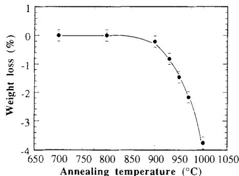
FIG. 5. Dependence of the weight loss before and after annealing on the annealing temperature of the  $(\text{Pb}_{0.7}\text{Cu}_{0.3})\text{Sr}_2(\text{Ca}_{0.5}\text{Y}_{0.5})\text{Cu}_2\text{O}_{7+\delta}$  samples.
