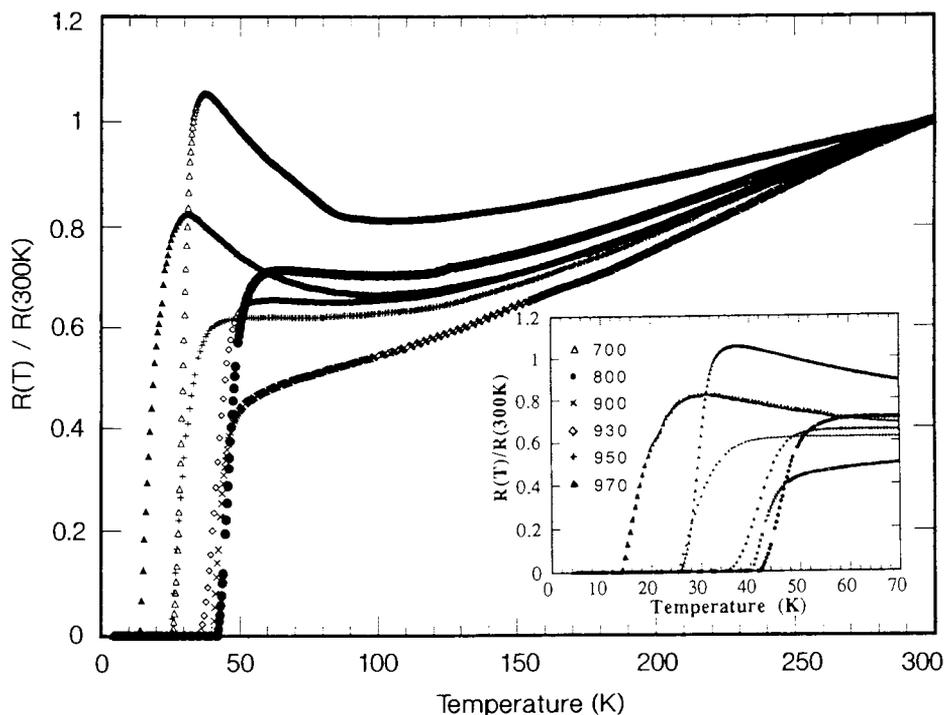
FIG. 2. Temperature dependence of the normalized resistance of the  $(\text{Pb}_{0.7}\text{Cu}_{0.3})\text{Sr}_2(\text{Ca}_{0.5}\text{Y}_{0.5})\text{Cu}_2\text{O}_{7-\delta}$  samples annealed at the temperatures of 700, 800, 900, 930, 950, and 970°C.
