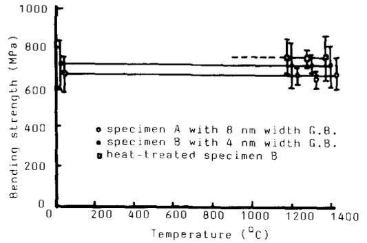
FIG. 4. The dependence of bending strength on temperature of  $\text{YL-Si}_3\text{N}_4$  ceramics with different GB widths.
