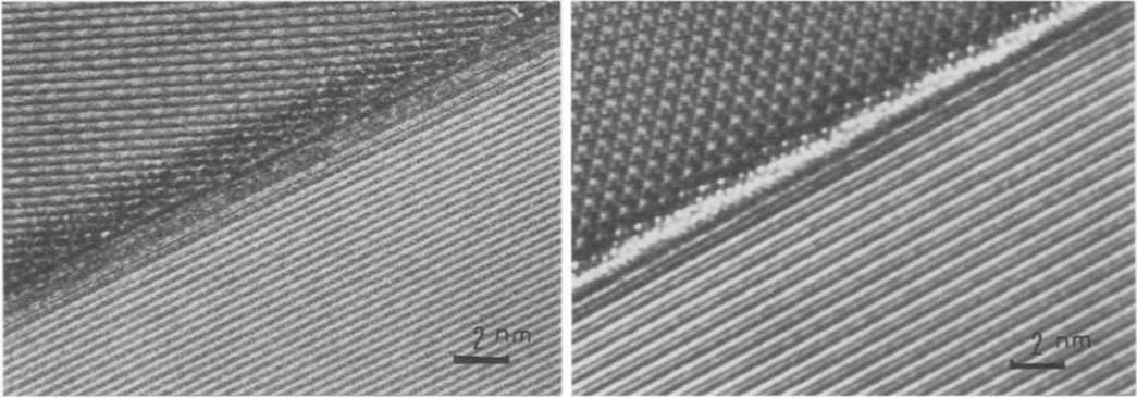
FIG. 6. HR-TEM picture of YL-Si<sub>3</sub>N<sub>4</sub> ceramics with different GB widths.
