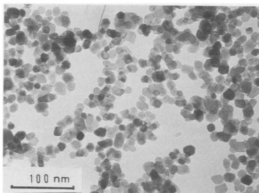
FIG. 3. A TEM micrograph, showing superfine  $ZrO_2$  powder stabilized by  $Y_2O_3$  and synthesized by a coprecipitation method.
