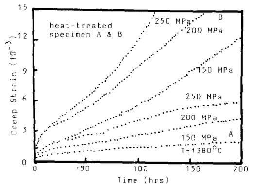
FIG. 5. The dependence of high temperature creep resistance of  $\text{YL-Si}_3\text{N}_4$  ceramics on different GB widths.
