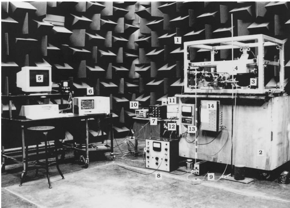
Figure 13. The chain testing hardware. 1, Frame; 2, hydraulic table; 3, hysteresis brake with coupler; 4, unislide table; 5, Compaq 386/20e with DAS-20; 6, HP analyzer; 7, electronic filters; 8, microphone amplifier; 9, microphone power supply; 10, oscilloscope; 11, current source; 12, power supply; 13, TSU tension readout; 14, strain gauge amplifier.
