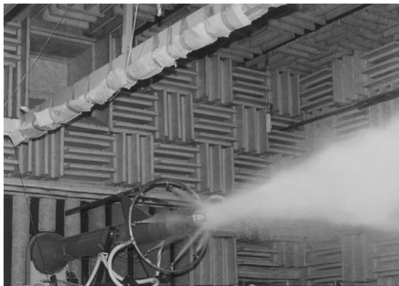
Figure 3. Noise reduction for high speed jets by means of water injection.
