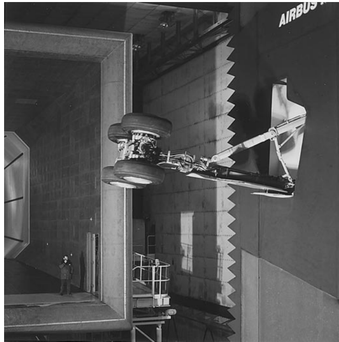
Figure 9. Full scale A 320 landing gear in the DNW for airframe noise studies.
