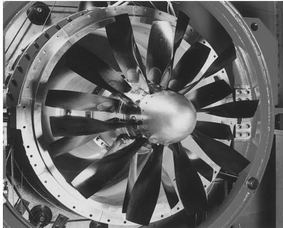
Figure 2. New counter-rotating 1 m model test stand at DLR, Cologne.
