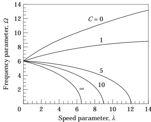
Figure 2. The frequency parameter  $\Omega$  in the fundamental mode for  $K = 1$  ( $\nu = 0.3, M = 5$ ).
