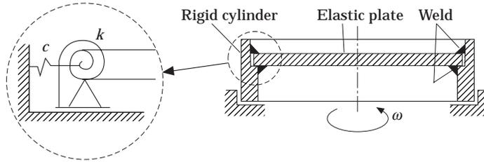
Figure 1. A circular plate supported elastically around its edge.
