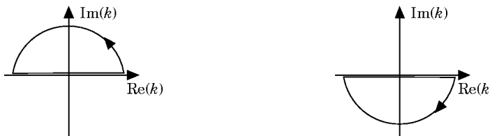
Figure 2. (a) Contour of integration in case of I_0 and I_+ ; (b) contour of integration in case I_- .
