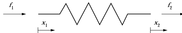
Figure 1. Spring element with nodal displacements x_1 and x_2 and nodal forces f_1 and f_2 .
