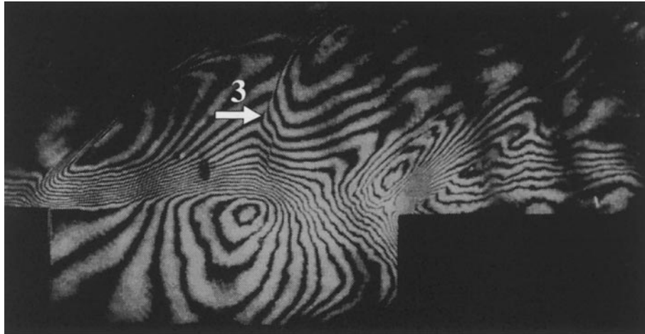
Figure 3. Holographic interferometry record of convecting vortex and Type 3 wave.
