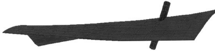
Figure 22. LPT wired assembly 7; cyclic symmetric sector (one blade and the associated wire portion).
