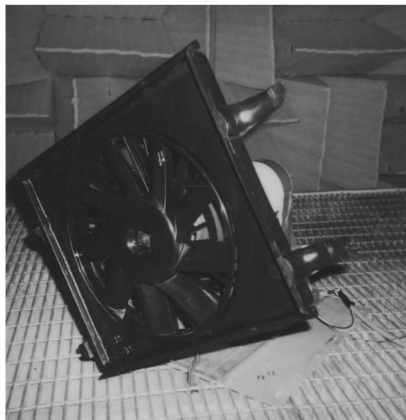
Figure 8. Experimental set-up for Type B fan with a shroud.
