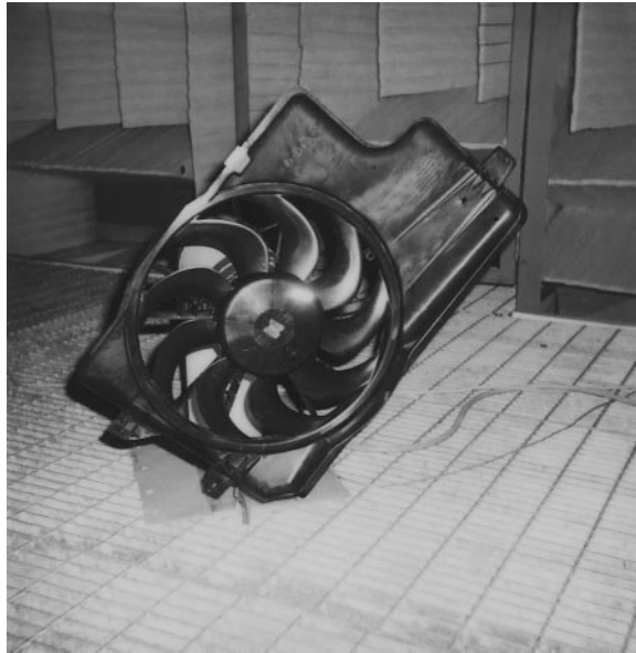
Figure 3. Experimental set-up for Type A fan with a shroud.
