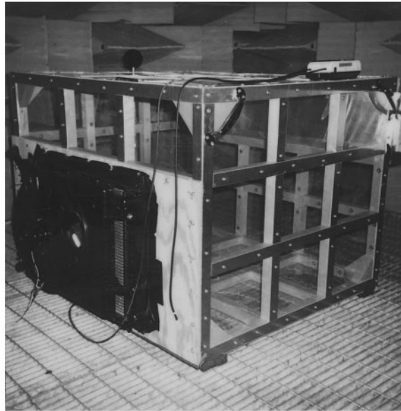
Figure 2. Experimental set-up of a cooling fan assembly mounted on a wood-framed box covered with Mylar sheet.
