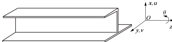
Figure 1. Beam co-ordinate system and displacement conventions.
