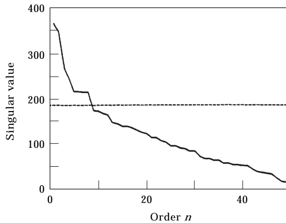
Figure 5. The singular spectrum of raw time series measured from the normal operating condition. The window length is 50 and the lag is 1.
