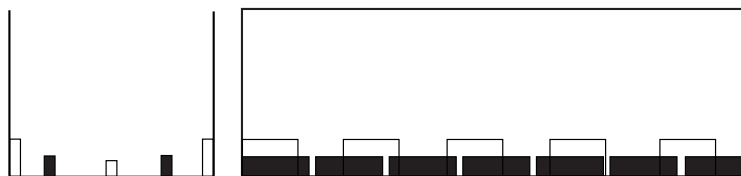
Rigid ground + Absorbing walls + Rigid restraints + Absorbing central reservation barrier (M15)
