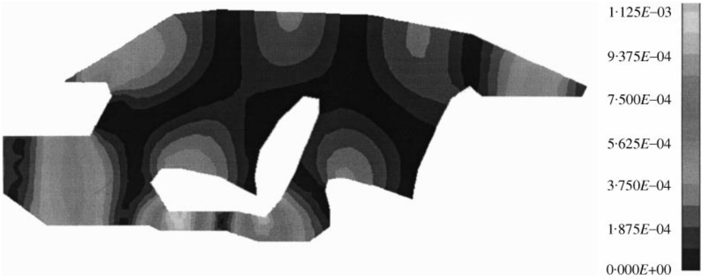
Figure 21. Velocity in car enclosure ( x direction/amplitude) at 350 Hz by initial mesh.
