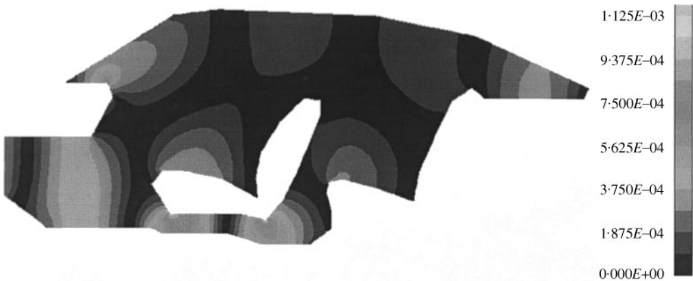
Figure 22. Velocity in car enclosure (x direction/amplitude) at 350 Hz by optimal mesh.
