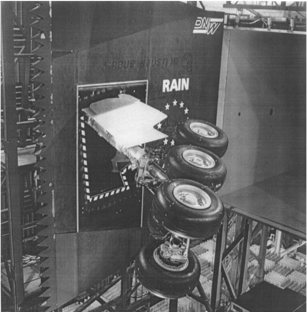
Figure 10. Aeroacoustic study of a full-scale A340 landing gear in the DNW wind tunnel.
