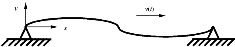
Figure 1. Axially accelerating string problem.
