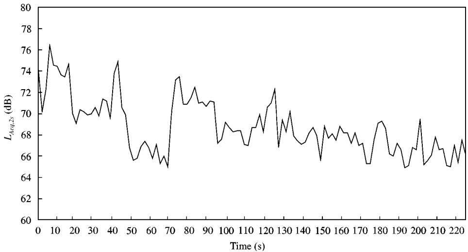
Figure 1. A-weighted sound pressure level inside a Mk 3 coach running at approximately 140 km/h.
