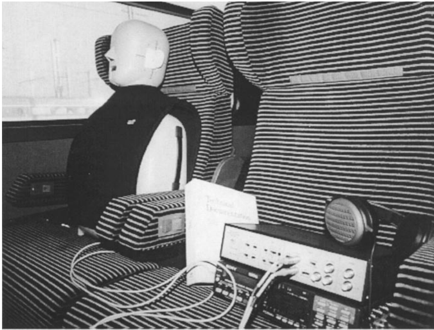
Figure 1. The acoustic head in the first floor of TGV Duplex.
