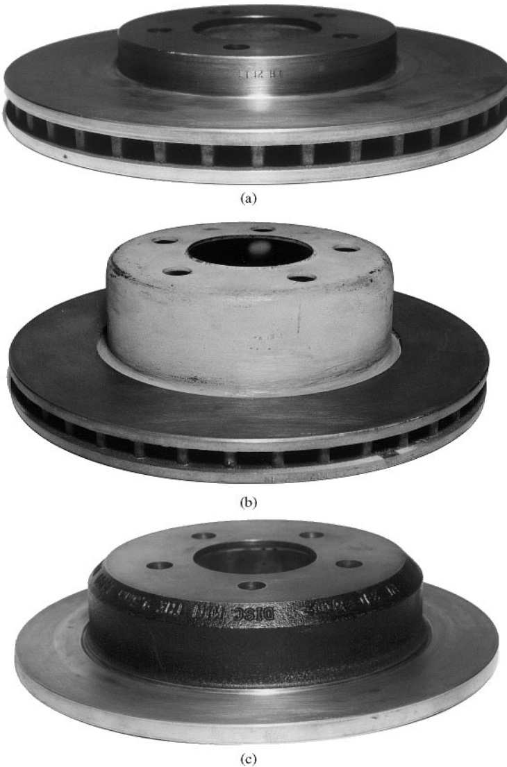
Figure 1. Photographs of typical (a) shallow-hat ventilated, (b) deep-hat ventilated, and (c) solid core brake rotors having different disk and hat element dimensions.
