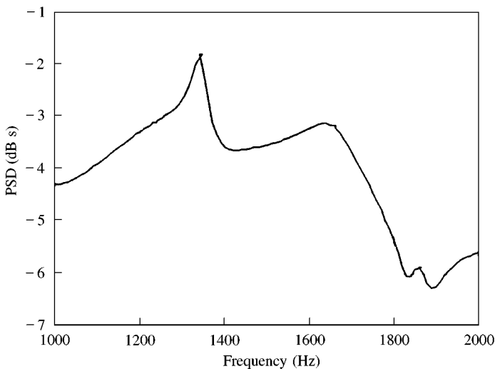
Figure 15. Spectral content of signal from faulty bearing (groove: 2.0 mm).
