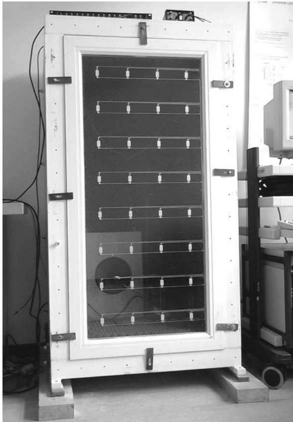
Figure 3. Experimental set-up: glass plate covered by an array of 4 \times 8 piezoelectric patches.
