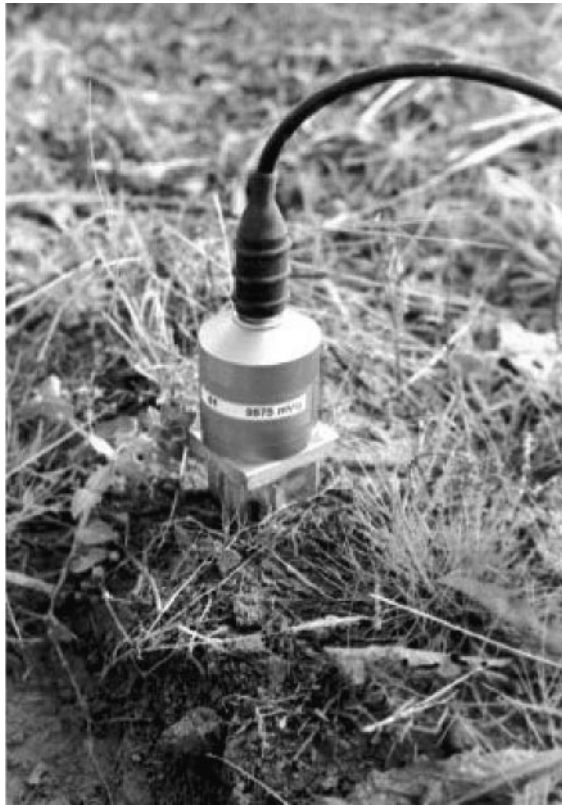
Figure 7. Seismic accelerometer mounted on an aluminium stake.
