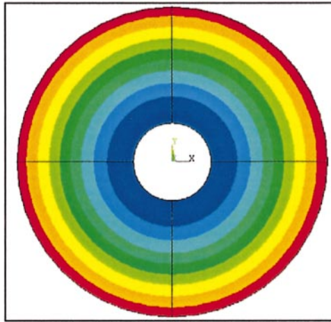
Figure 3. The mode shape of the second natural frequency (296.04 Hz).
