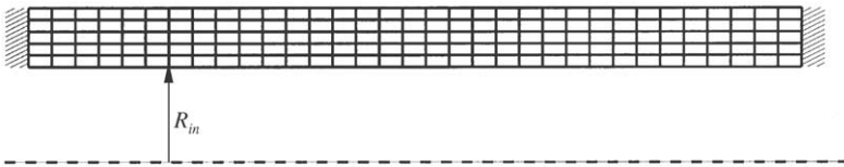
Figure 4. Finite element mesh for the clamped tube section. In the actual computation, there are 500 elements in the axial direction and five in the radial direction.
