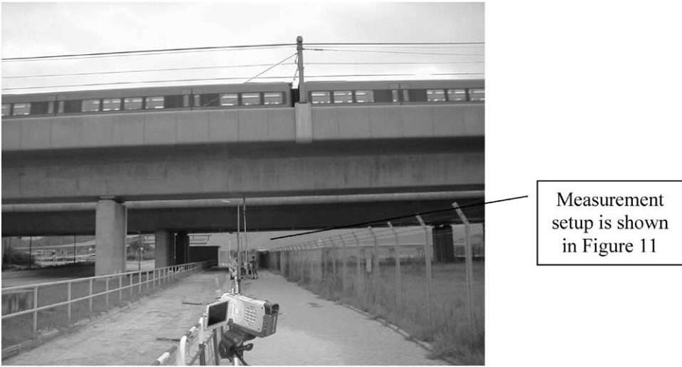
Photo 1. Measurement locations of vibration and structure-borne noise measurement of the concrete railway viaduct.
