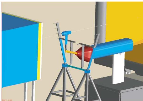
Figure 3. Test of NLR model turbofan in the DNW-LLF.
