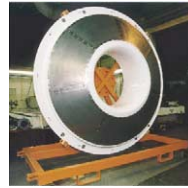
The Negatively Scarfed Intake (Scale model flare manufactured by RR).
