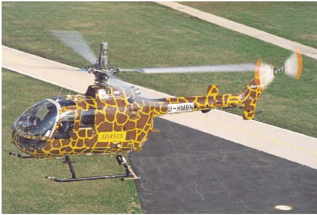
Figure 22. The BO 105 IBC demonstrator used for flight tests.
