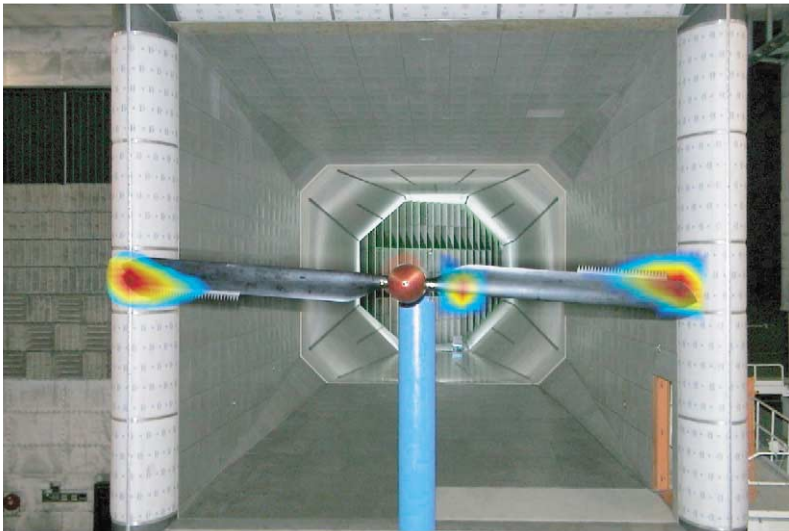
Figure 17. Acoustic image of model wind turbine at 8000 Hz, obtained with ROSI.
