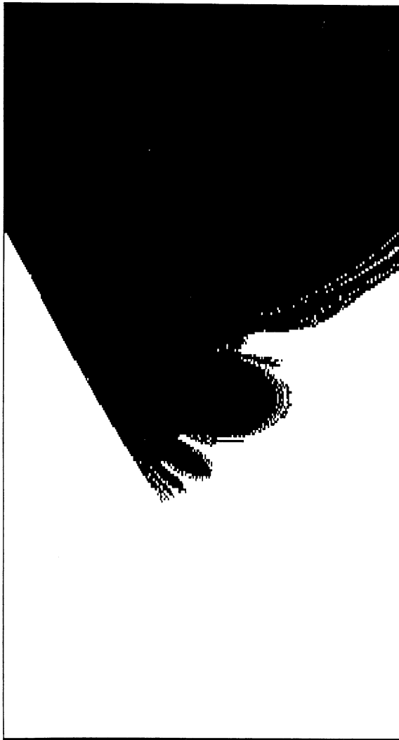
Figure 9. Transient time map in (A_f, \Omega) parameter space. For this diagram the range of (A_f, \Omega) correspond to Figure 5 and W(0) = \dot{W}(0) = 0 . Maximum number of forcing cycles ( m=20 ) and a failure criterion is chosen at W_{max}=1 . White indicates safe basin; black indicates unsafe basin.
