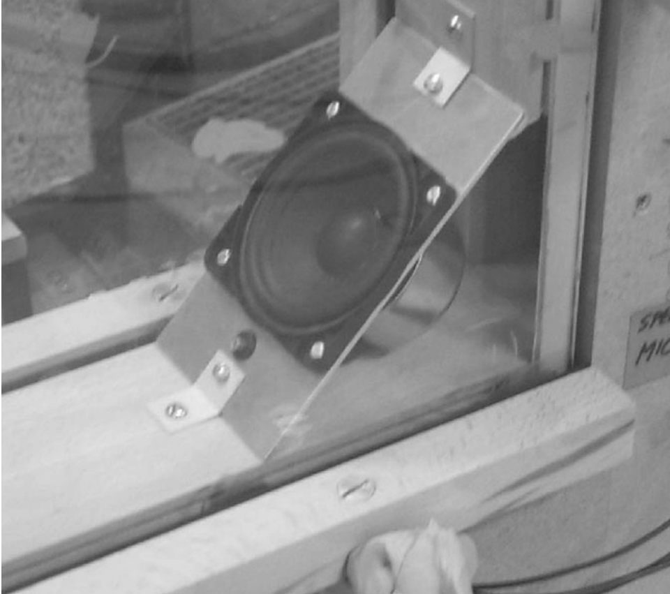
Fig. 2. Control speaker in the cavity between the panes. A microphone is mounted adjacent to the speaker.
