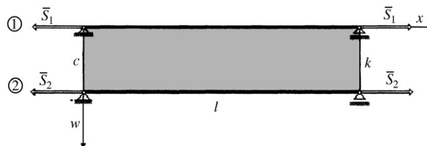
Fig. 2. The physical model of an elastically connected double-string system analyzed for free motions.
