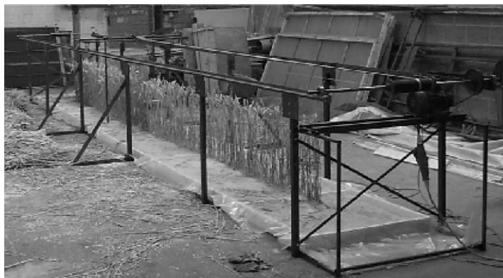
Fig. 5. Experimental set-up for dynamic crop density measurements.
