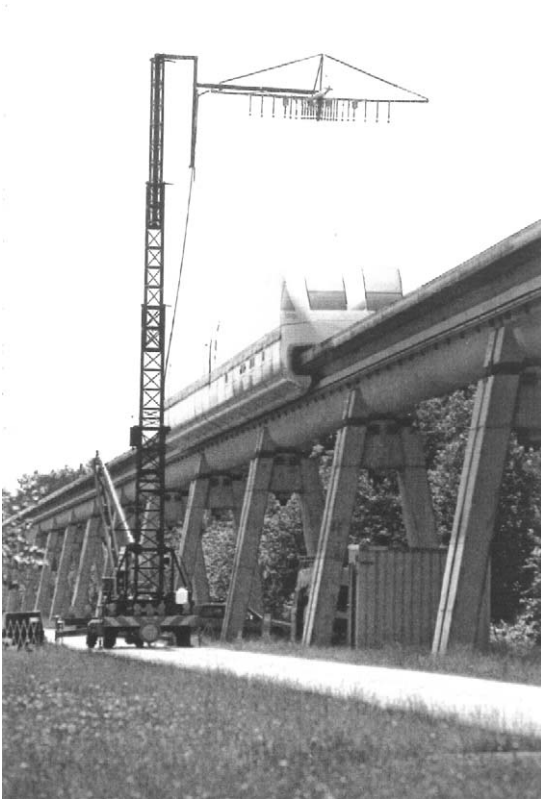
Fig. 1. Turbulent boundary layer sources on the roof of a TR07 vehicle.
