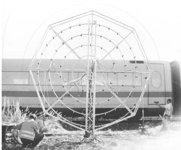
Fig. 3. Spiral array developed at DB-AG.
