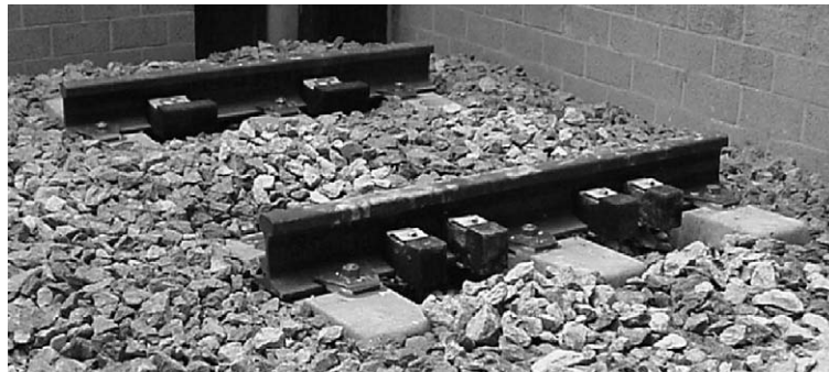
Fig. 20. The short ballasted rail track test set-up.
