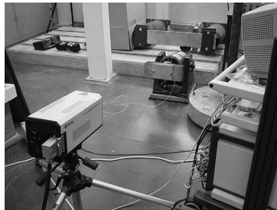
Fig. 12. Set-up of laser Doppler vibrometer.
