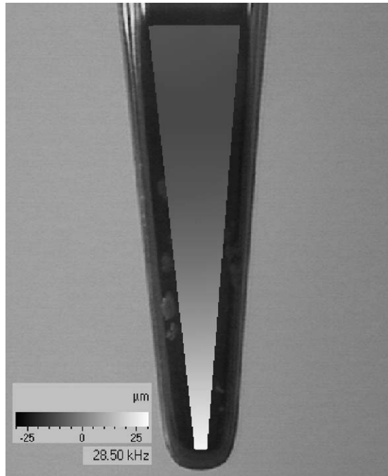
Fig. 3. Scanning laser vibrometer scan of a TFI-3 magnetostrictive scaling tip (Dentsply Preventive Care, York, PA, USA). Vibration data are superimposed upon a video image of the insert probe.
