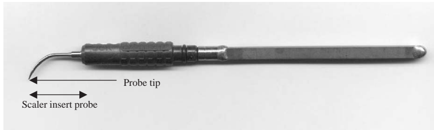
Fig. 1. A dental ultrasonic scaler insert showing the metal probe used for tooth debridement.
