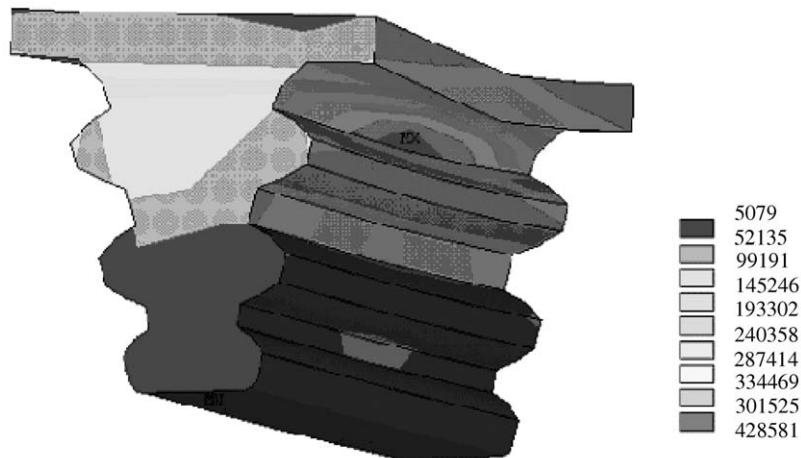
Fig. 27. Stress distribution of the blade root from the harmonic analysis (r.p.m. = 4338).
