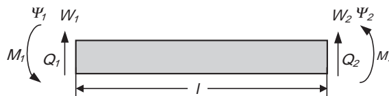
Fig. 1. Sign convention for the finite Timoshenko-beam element.
