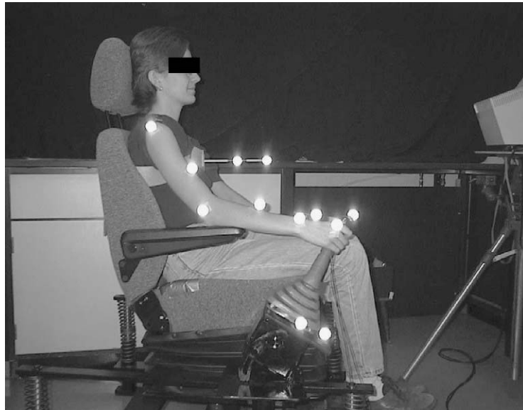
Fig. 3. Subject and retroreflective marker placement in excavator cab/joystick mock-up.
