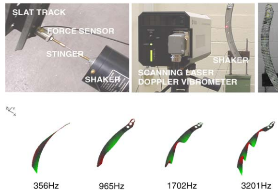
Fig. 8. Force (input) measurement with shaker, stinger and impedance head attached to the slat track (top, left). Velocity measurement with SLDV in grid of 352 points (top, middle & right). Some mode shapes of the slat track with bending and torsional behavior (bottom).
