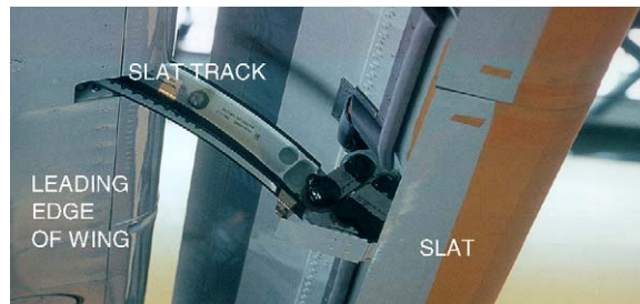
Fig. 7. A Slat track mounted in the wing of an Airbus320 aircraft.
