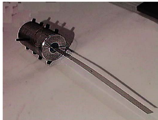
Fig. 1. The rotating beam with the piezoceramic actuator.
