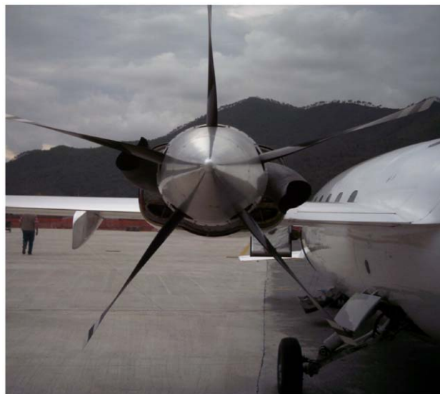
Fig. 7. P180 ground noise test for exhaust shape and orientation optimisation.
