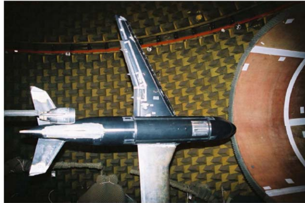
Fig. 4. Fan noise test in ONERA CEPR 19: ROSAS model and TPS nacelle, RFN layout.
