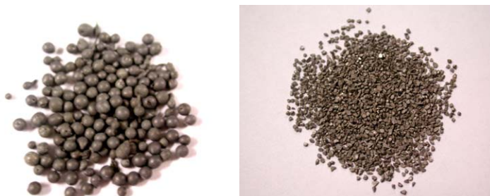
Fig. 2. Metal particles as damping material: lead particles (left) and tungsten carbide particles (right).
